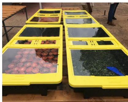
Fig. 20: Dehytray™ - loaded with tomato slices and blanched leafy vegetables
