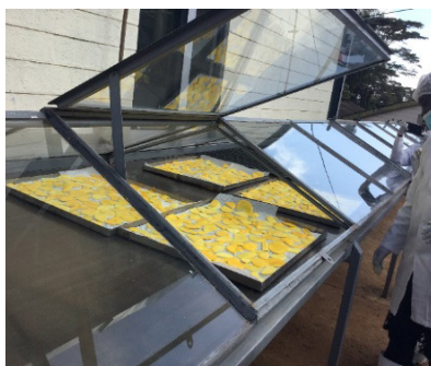
Fig. 19: Tunnel Solar Dryer - loaded with mango chips
