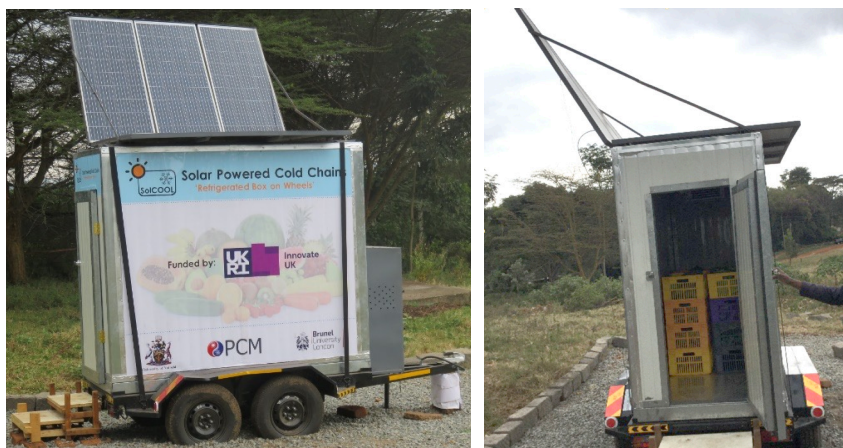
Fig. 16: A refrigerated box on wheels – a possible low-cost alternative to refrigerated trucks
