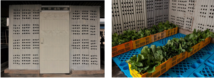
Fig. 15: The improved charcoal cooler with fibreglass encasing – the appearance outside and inside
